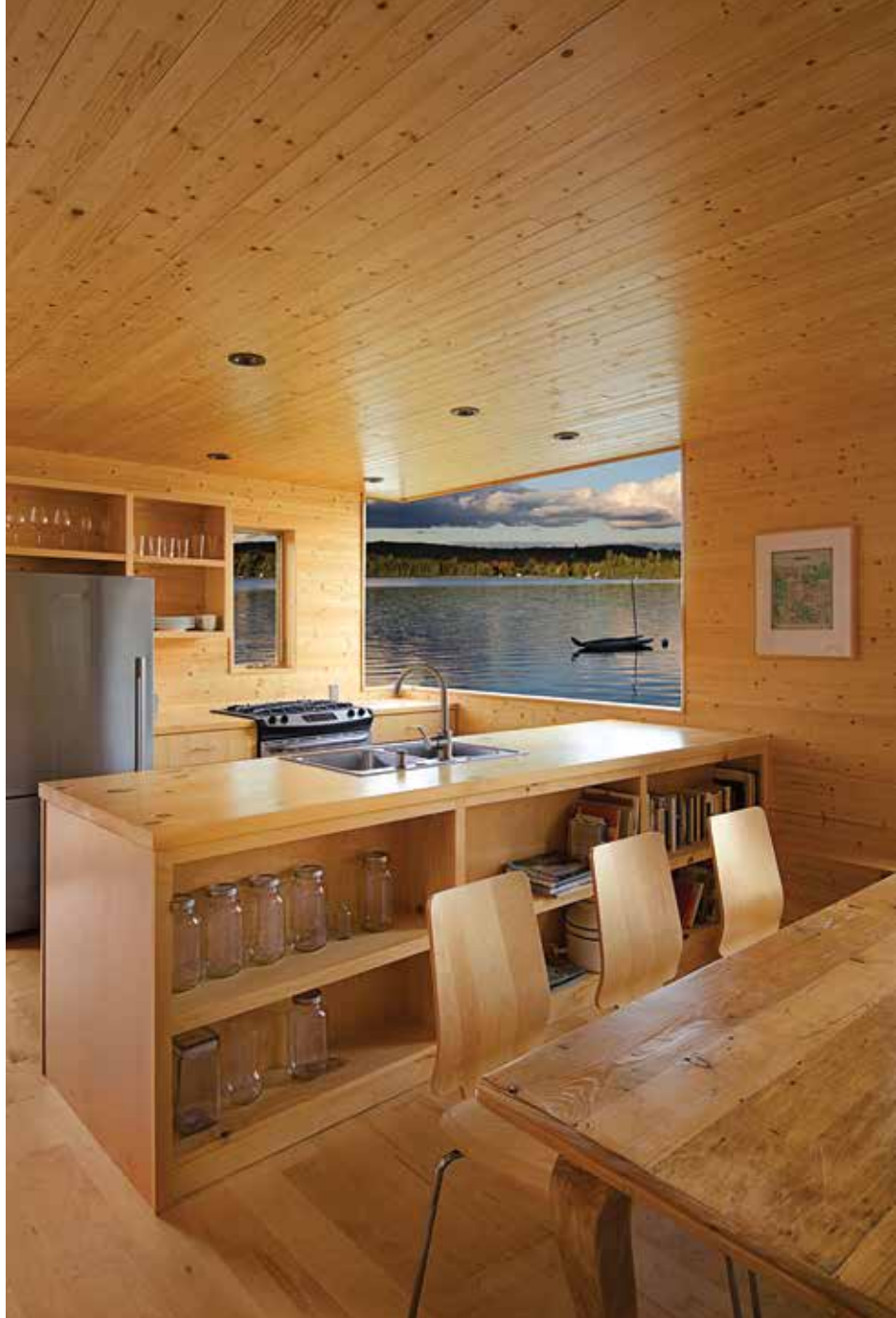
No sheetrock or other drywall construction is used in the camp because it is designed to weather severe changes in temperature, which cause expansion and contraction of materials throughout all four seasons, especially during the wintertime when the building does not see use.
